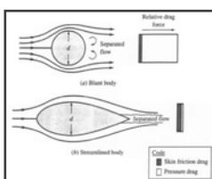
The trailing edge is the edge where air comes back together. Theoretical models often use very sharp points, but carbon doesn't like sharp angles, so in actual product, a slightly rounded trailing edge gives the best results for strength. A cylindrical airfoil has a rounded trailing edge and creates a lot of turbulence.
