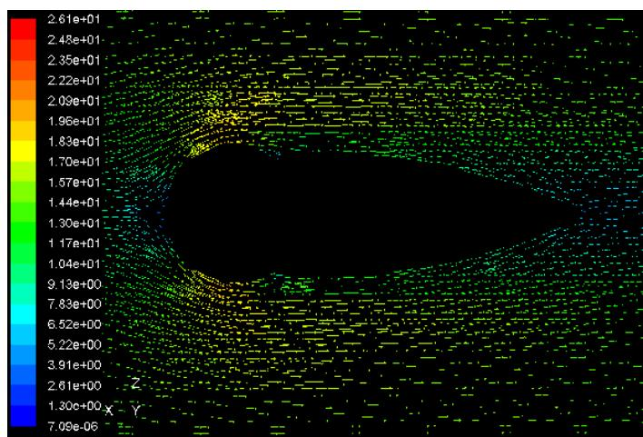
Fig. 2 – CFD model of flow around tire and aerodynamic rim at 50km/h rotation and wind speed
