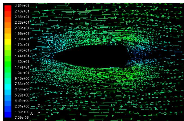
Fig. 9 – CFD model of a 50km/h rotation and wind speed showing small area of trailing edge separation (blue)
